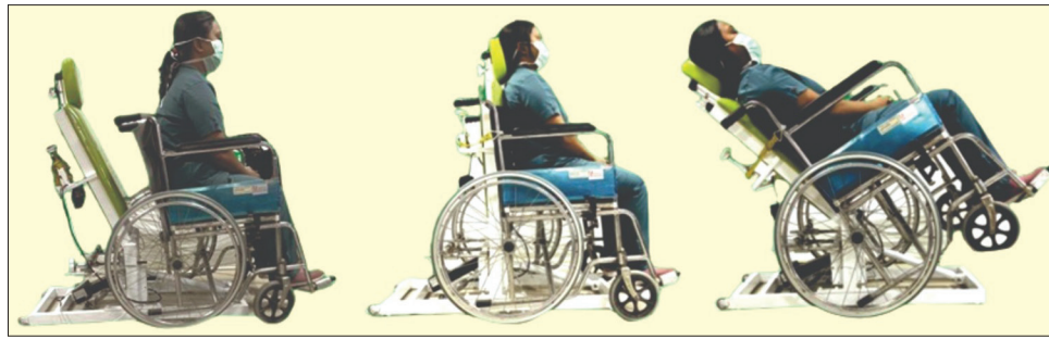
Figure 2: Recliner being placed under wheelchair and tilting the wheelchair to enable the dentist to provide dental care at wheelchair itself
