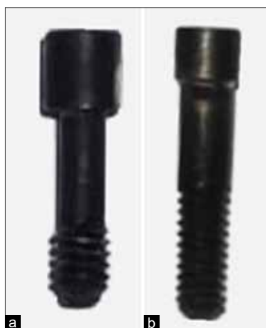
Figure 2: Abutment screws with plasma nitriding treatment (a) genesis aktiv implant system abutment screw (b) bredent implant system abutment screw
