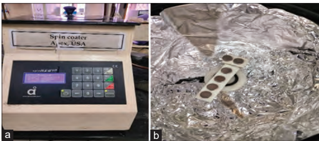
Figure 4: (a) SPIN coating machine, manufactured by APEX, USA. (b) Discs into the coating machine during coating procedure
