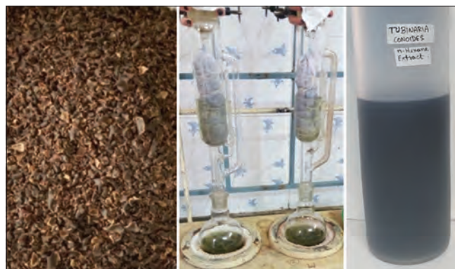
Figure 1: Soxhlet extraction of T. conoides in n-hexane. T. conoides : Turbinaria conoides
