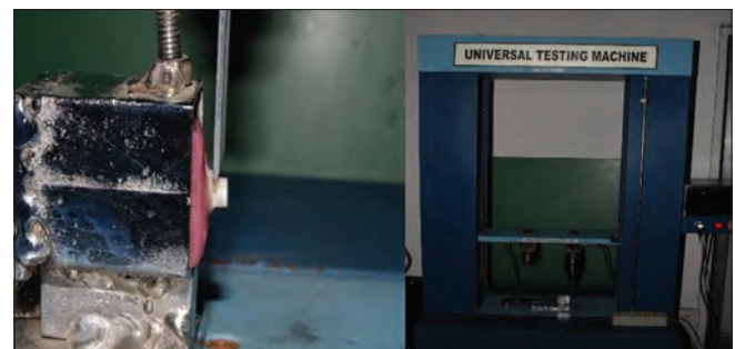
Figure 3: Prepared sample placed in the universal testing machine for shear bond strength
