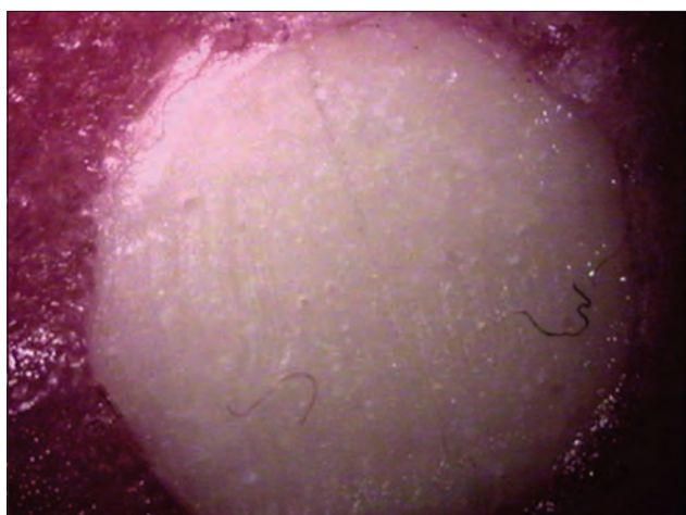
Figure 4: Adhesive failure pattern of Group A at ×10 magnification by a stereomicroscope
