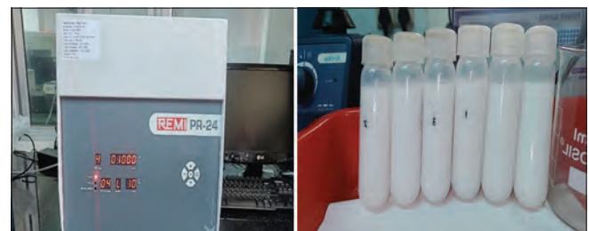
Figure 1: REMI centrifugation machine and centrifuged test tubes during centrifugation of BN solution. BN: Boron nitride
