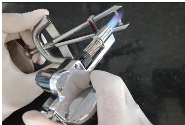
Figure 5: Heating the threaded screws of the instrument using a flame torch
