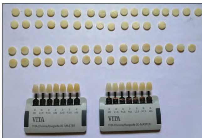
Figure 4: Specimens and shade guides on the white background used for color measurement
