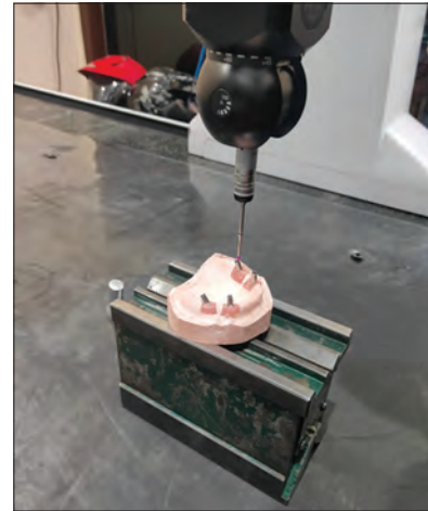
Figure 11: Stone cast being measured with standard abutments in place on the CMM machine. CMM: Coordinate measuring machine
