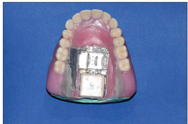
Figure 2: Vacuum-packed denture tracker with thermoforming materials
