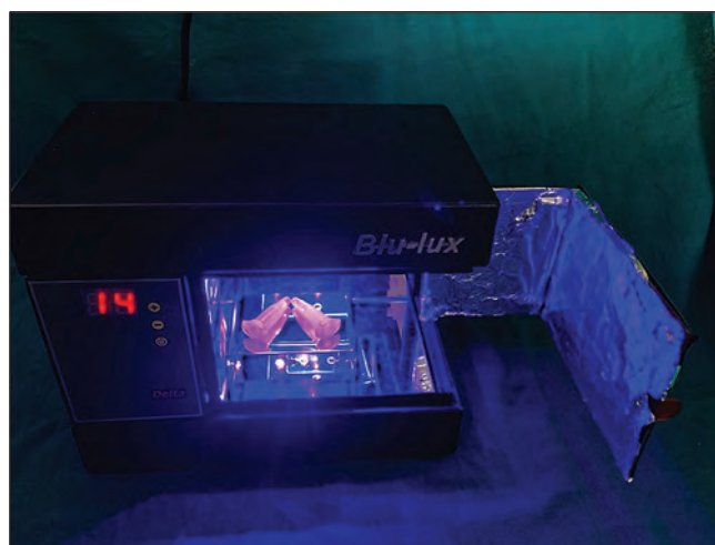
Figure 5: Exposure of sample solutions to blue LED light after application of viability dye, PMAxx. LED: Light-emitting diode
