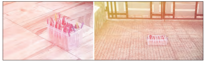
Figure 1: Exposure of conventional and POSS-modified samples to UV radiations (day light). POSS: Polyhedralsilsesquioxanes, UV: Ultraviolet
