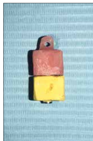
Figure 2: O-ring connector in place after processing the experimental base (Male connector)
