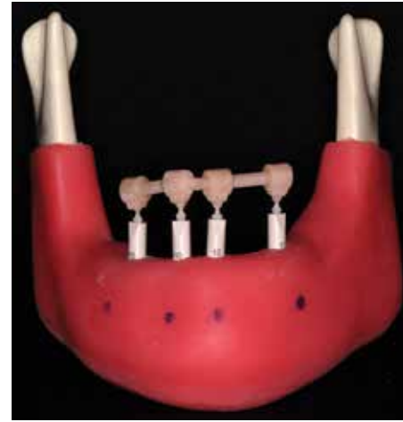
Figure 3: Master model with the device attached to the scan bodies (SD). SD: Scan device
