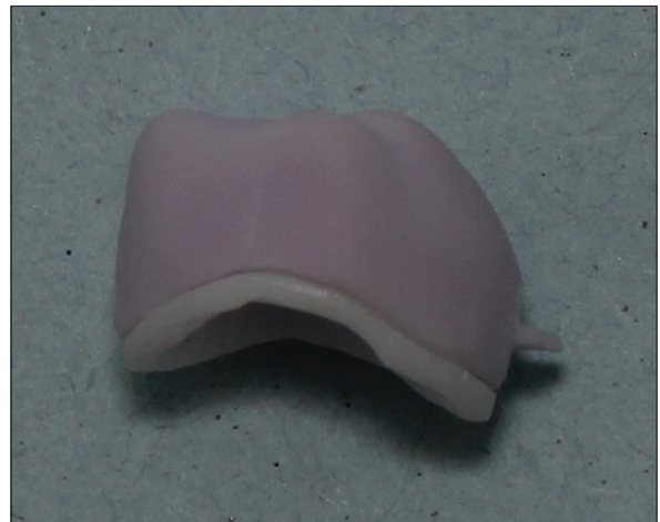
Figure 2: Fusing the coping and veneer using IPS e.max Crystal/Connect material
