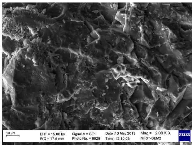
**Fig. 4** SEM of deglazed surface (Original  $\times 2000$ )
