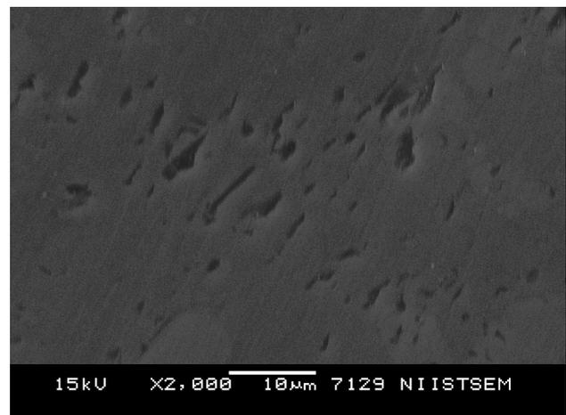
**Fig. 9** SEM of surface polished with adjustment kit + diamond wax (Original  $\times 2000$ )
