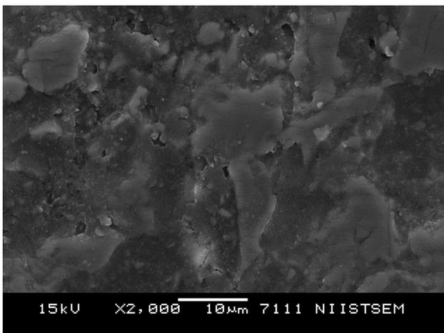
**Fig. 7** SEM of surface polished with diamond wax (Original  $\times 2000$ )
