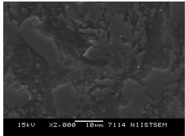
**Fig. 8** SEM of surface polished with wheel + diamond wax (Original  $\times 2000$ )
