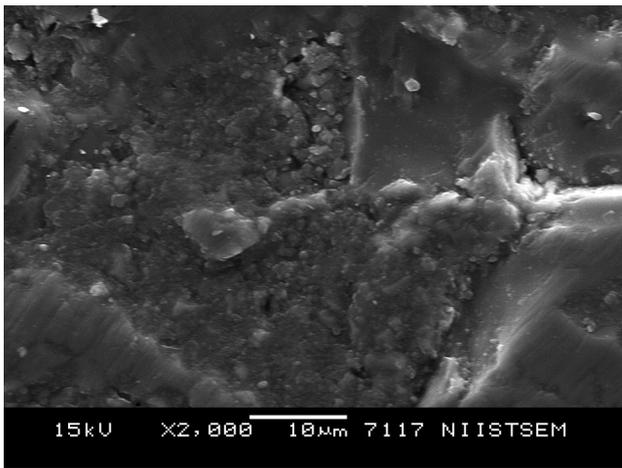
**Fig. 5** SEM of surface polished with polishing wheel (Original  $\times 2000$ )
