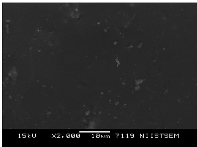
**Fig. 3** SEM of glazed surface (Original  $\times 2000$ )
