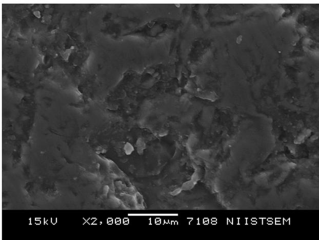
**Fig. 6** SEM of surface polished with adjustment kit (Original  $\times 2000$ )
