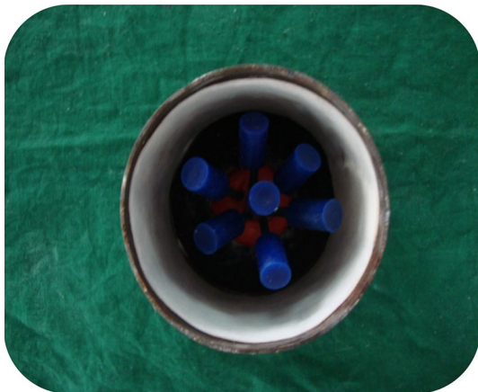
Fig. 3 Sprued wax patterns assembled in the casting ring
