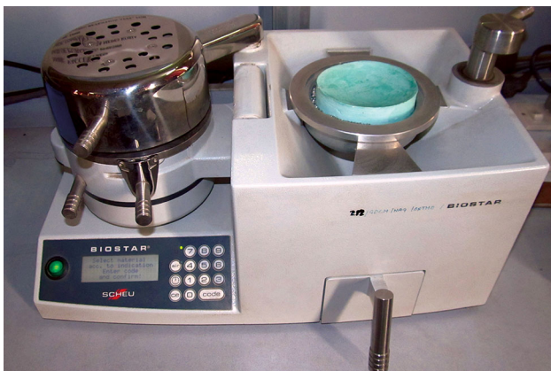
Fig. 3 Concave stone-form placed in heat and pressure molding machine
