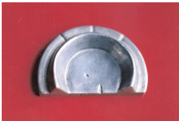
Fig. 2 Aluminum die simulating the maxillary edentulous arch
