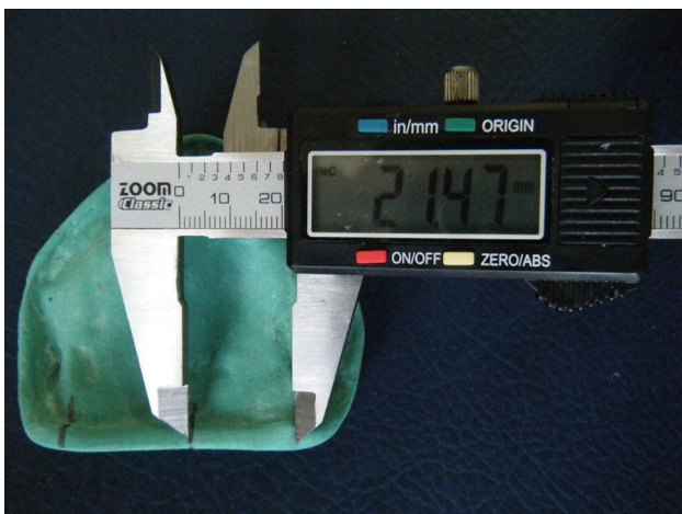
Fig. 1 Marking of the centre point for hook placement with the help of a vernier caliper
