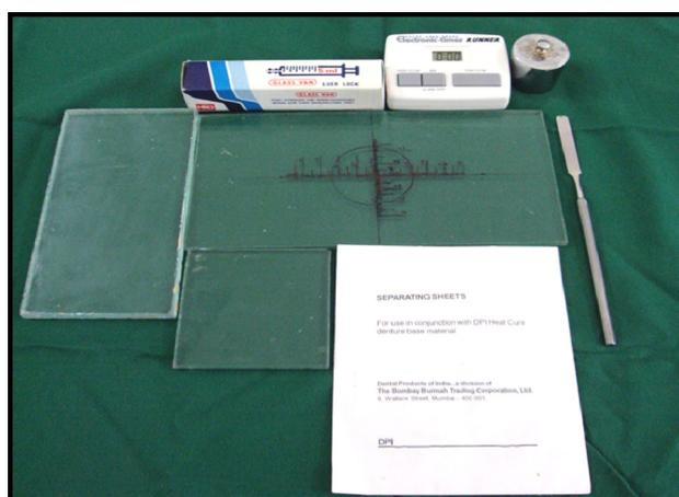
**Fig. 2** Glass plate, glass slab, stainless steel spatula, glass syringe, stop watch, 500 g weight for flow property
