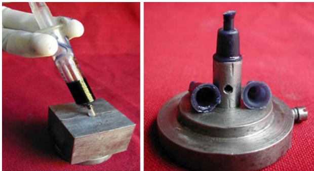
Fig. 3 Molten wax injected into the warmed assembly chamber and prepared wax pattern
