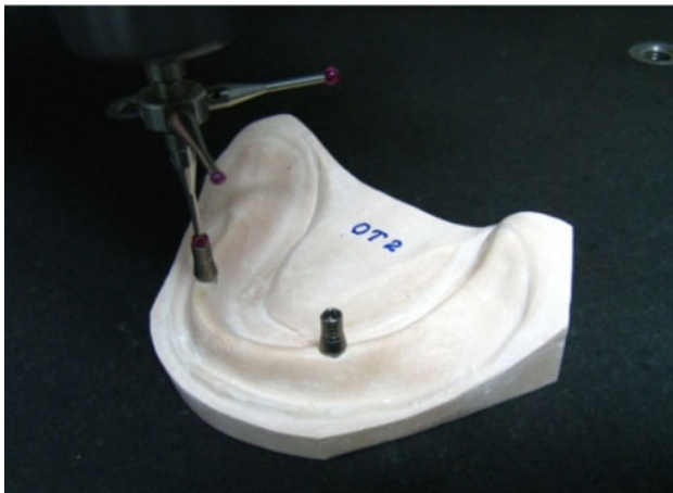
Fig. 6 Measuring coordinates on the open tray cast
