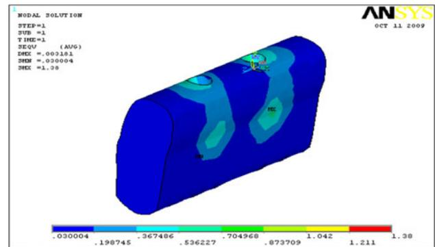
**Fig. 26** Stresses on cancellous bone zirconium–axial loading-model-3
