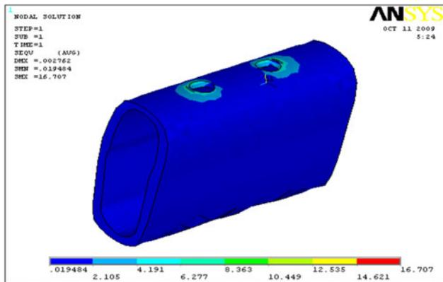
Fig. 10 Stresses on cortical bone-titanium-non-axial loading model-2
