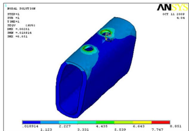
**Fig. 9** Stresses on cortical bone-titanium—non-axial loading-model-1
