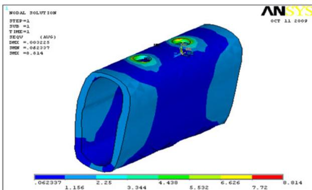
**Fig. 18** Stresses on cortical bone zirconium—axial loading-model-1
