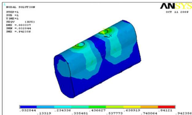
Fig. 12 Stresses on cancellous bone-titanium-axial loading-model-1
