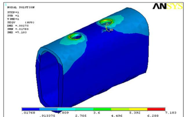
**Fig. 21** Stresses on cortical bone zirconium—non-axial loading-model-1
