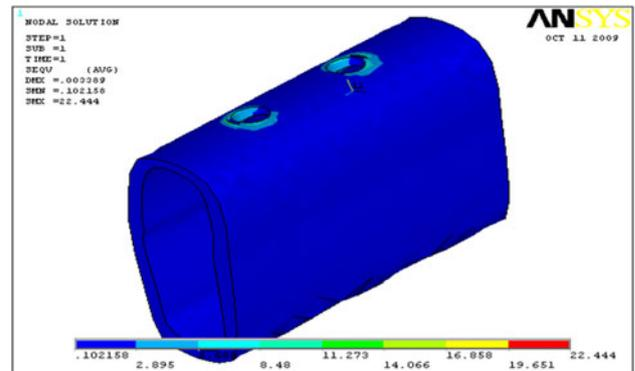
**Fig. 20** Stresses on cortical bone zirconium—axial loading-model-3
