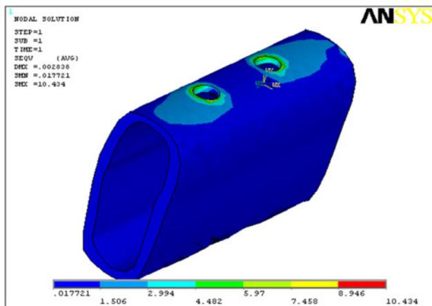
Fig. 11 Stresses on cortical bone-titanium-non-axial loading model-3
