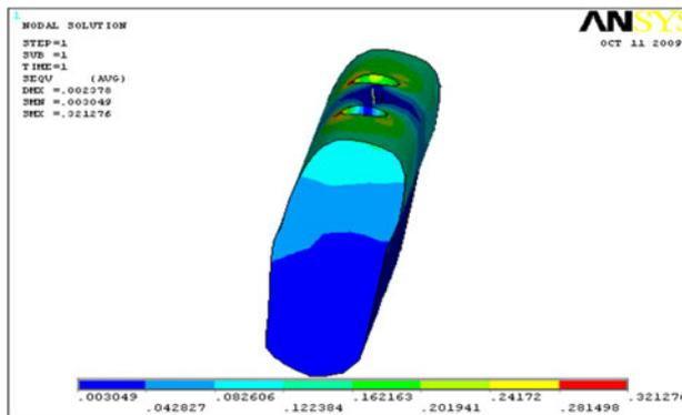
Fig. 15 Stresses on cancellous bone-titanium-non-axial loading-model-1
