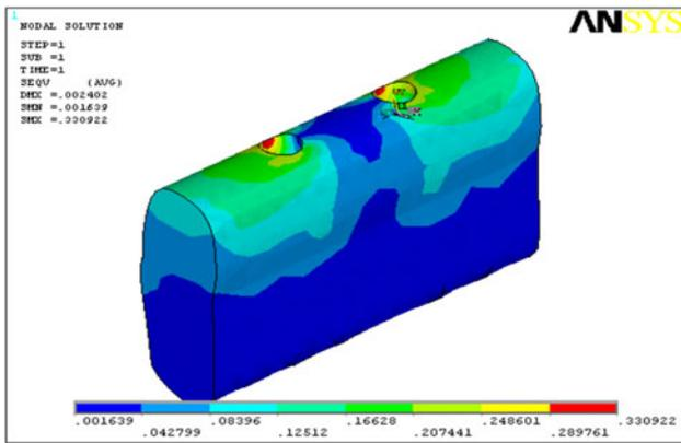
**Fig. 16** Stresses on cancellous bone—titanium—non-axial loading-model-2
