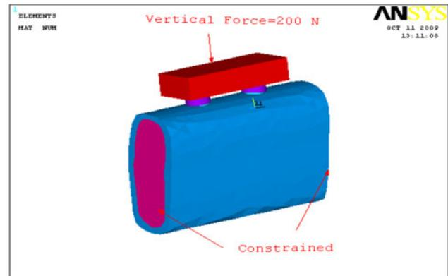
**Fig. 4** Assembly after application of boundary conditions—axial loading
