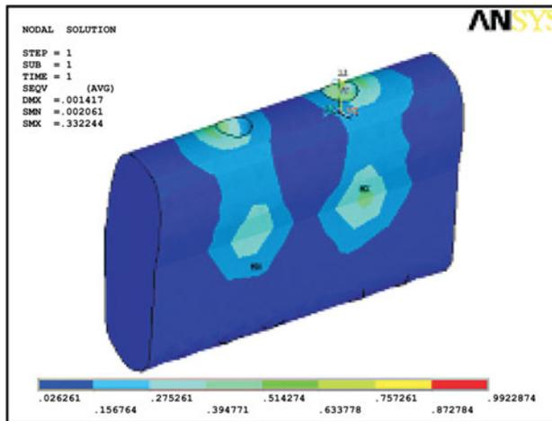
Fig. 13 Stresses on cancellous bone-titanium-axial loading-model-2
