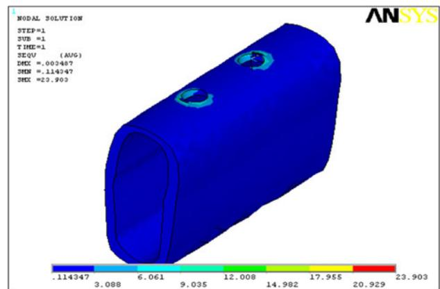
**Fig. 8** Stresses on cortical bone-titanium—axial loading-model-3
