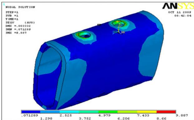
**Fig. 6** Stresses on cortical bone-titanium—axial loading-model-1
