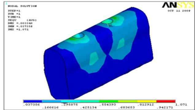
**Fig. 25** Stresses on cancellous bone zirconium–axial loading-model-2
