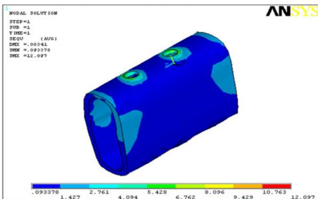
**Fig. 7** Stresses on cortical bone-titanium—axial loading-model-2
