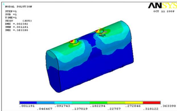
**Fig. 28** Stresses on cancellous bone zirconium–non-axial loading-model-2
