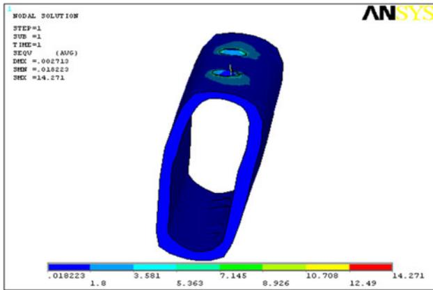
**Fig. 22** Stresses on cortical bone zirconium–non-axial loading-model-2
