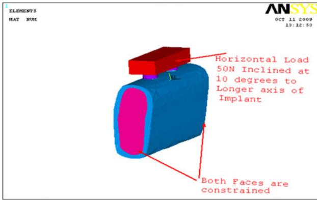
**Fig. 5** Assembly after application of boundary conditions—non-axial loading
