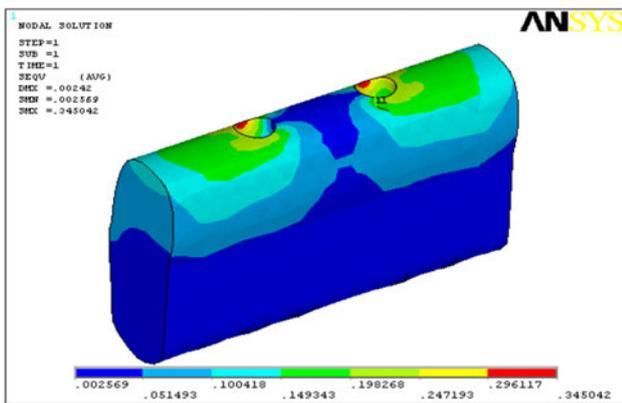
**Fig. 17** Stresses on cancellous bone—titanium—non-axial loading-model-3
