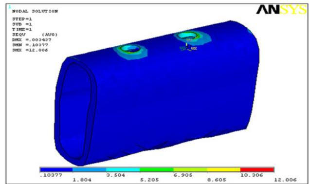
**Fig. 19** Stresses on cortical bone zirconium—axial loading-model-2
