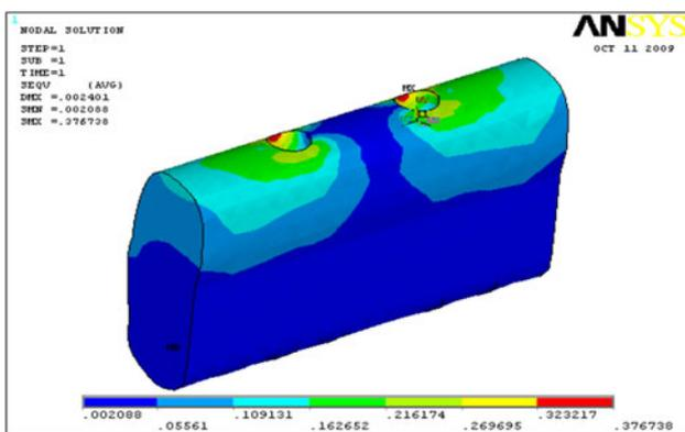
**Fig. 29** Stresses on cancellous bone zirconium–non-axial loading-model-3
