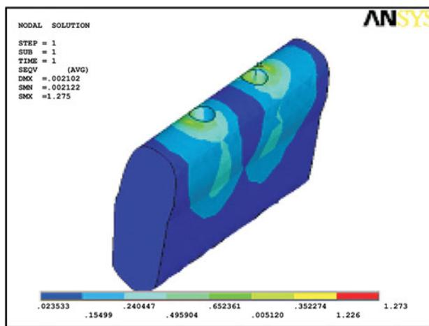
Fig. 14 Stresses on cancellous bone-titanium-axial loading-model-3
