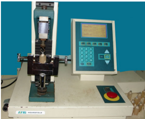
Fig. 3 Sample was mounted on Hounsfield universal testing machine and subjected to retentive test
