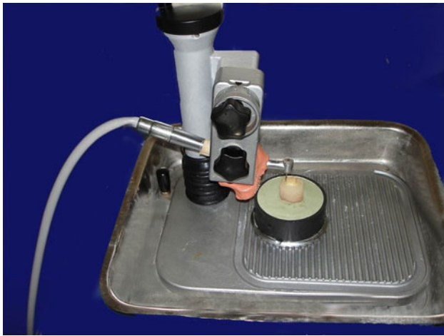
Fig. 1 Prepared tooth using Aerotor handpiece clamped to Kavo milling apparatus
