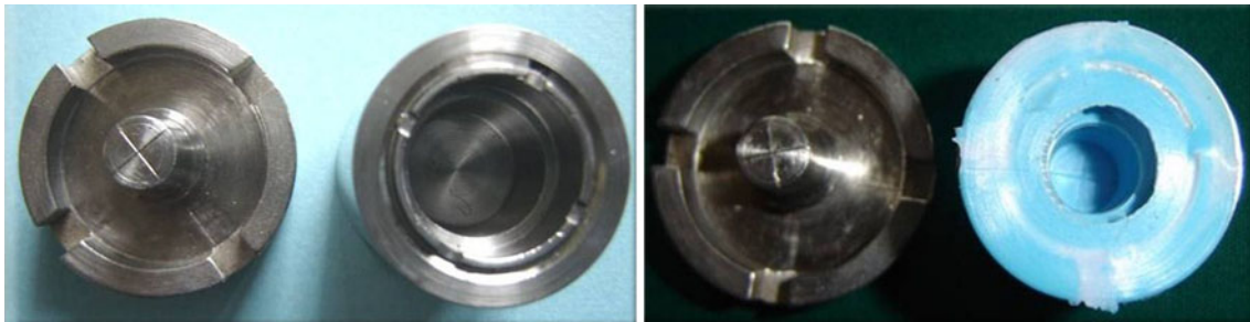
Fig. 3 Master metal die, impression tray and corresponding PVS impression
