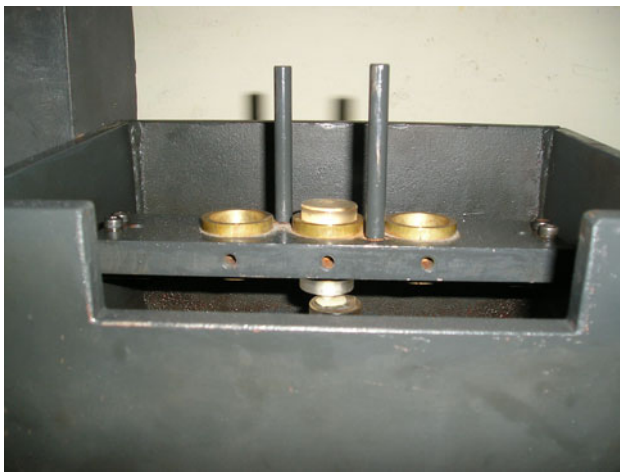
Fig. 5 Test specimens mounted on wear simulator-tooth specimen as upper member and ceramic specimen as lower member
