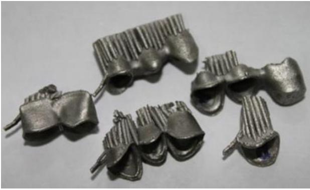
Fig. 2 Laser sintered crown and fixed partial denture copings before finishing
