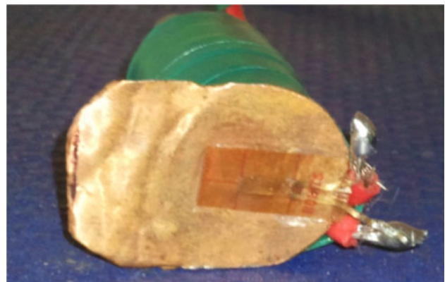
Fig. 3 Pressure transducer made of a tin chamber with a copper diaphragm to which a strain gauge is bonded
