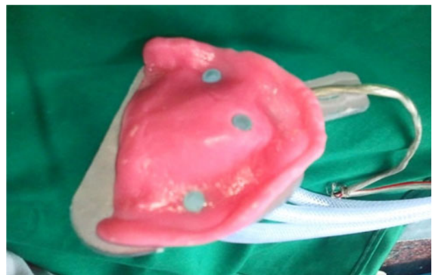
Fig. 2 Impression tray connected to tubes filled with distilled water
