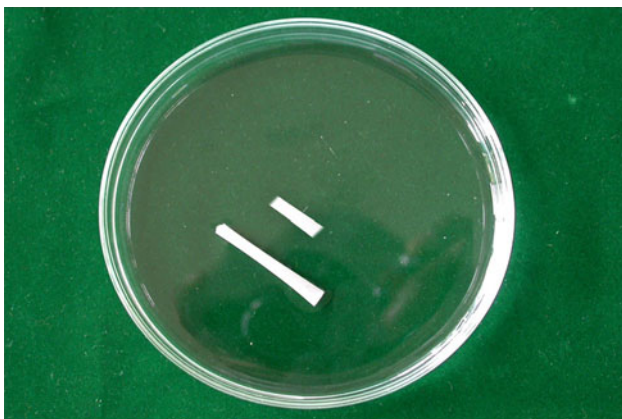
Fig. 8 Silane treatment of glass fibers
