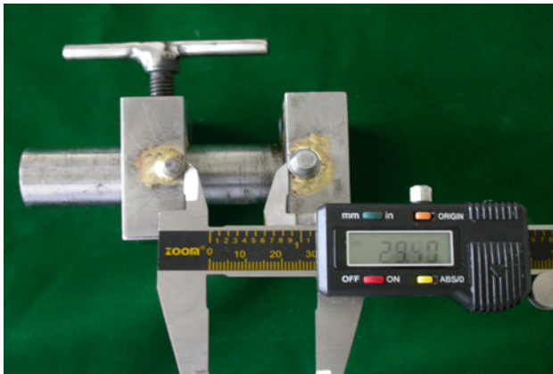
Fig. 5 Span of interim fixed partial denture being measured using a digital caliper
