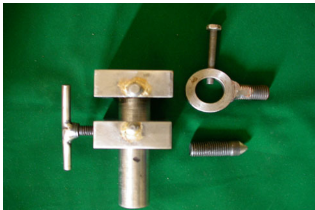
Fig. 1 Mounting Jig with stabilizing screw and loading device
