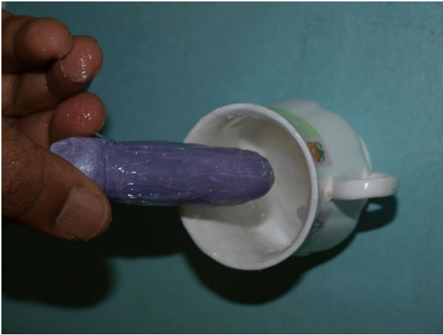
Fig. 3 Model dipped in silicone
