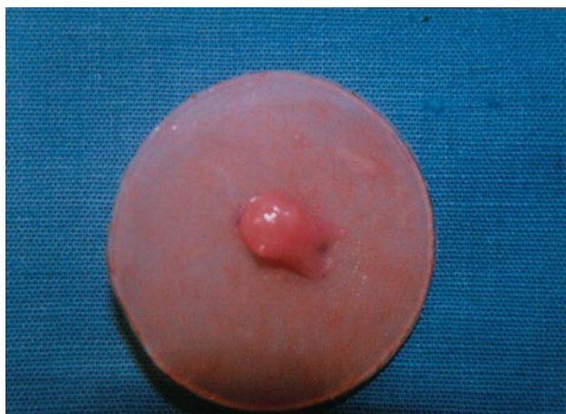
Fig. 8 Adhesive paste applied on the disk surface
