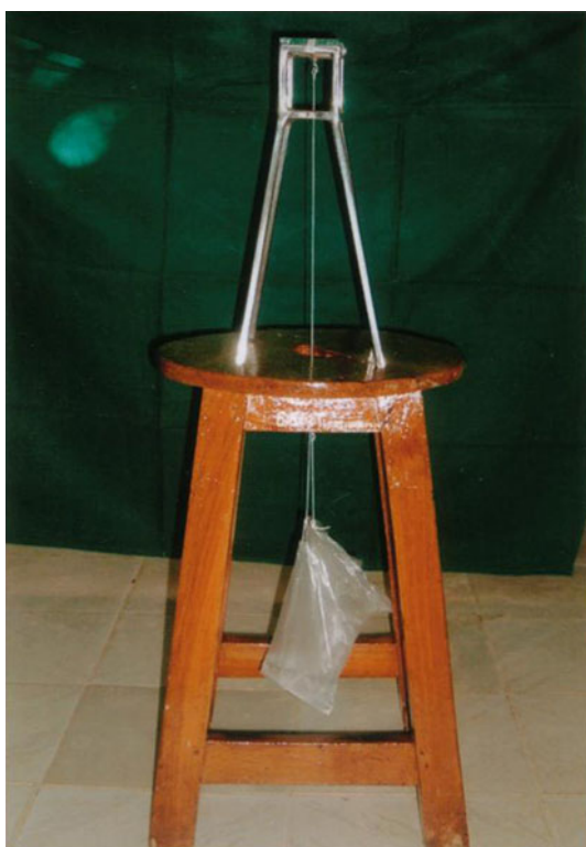
Fig. 5 Testing apparatus used to evaluate the adhesion of distilled water and artificial saliva
