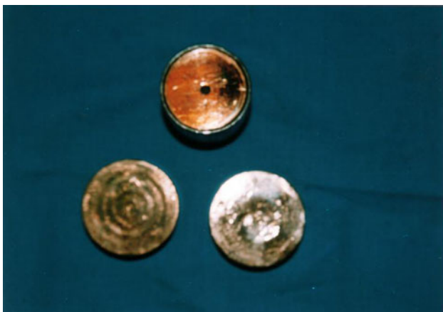
Fig. 1 Metal die with the bronze disks
