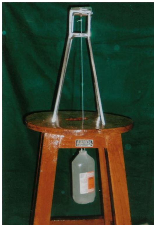
Fig. 6 Testing apparatus used to evaluate the adhesion of various test materials with and without artificial saliva
