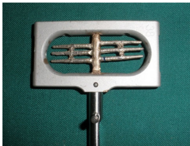
Fig. 4 Wax patterns coated with silver oxide on mounting frame
