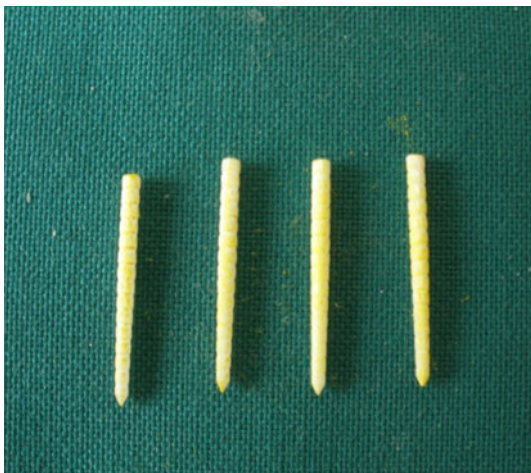
Fig. 6 Zirconia posts (Post sintering)
