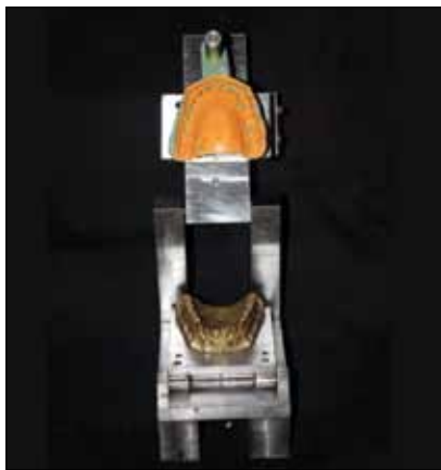
Figure 5: Group 3: Multiple mix technique utilizing heavy viscosity and low viscosity combination in custom trays
