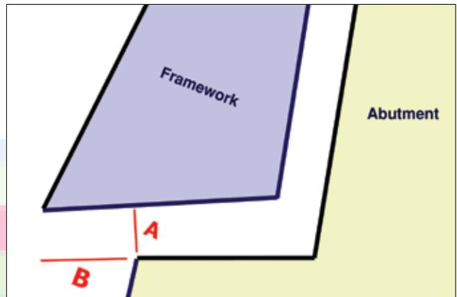
**Figure 4:** Schematic measurement of vertical (A) and horizontal (B) discrepancy after sectioning resin block longitudinally through the center
