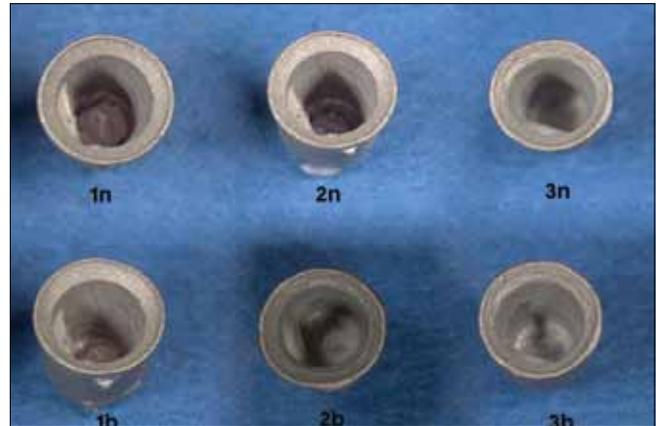
**Figure 2:** Metal copings fabricated using three different techniques (1: waxing using burn-out, 2: waxing on the impression coping, and 3: conventional waxing) and two types of alloy (n: gold alloy, b: base metal alloy)
