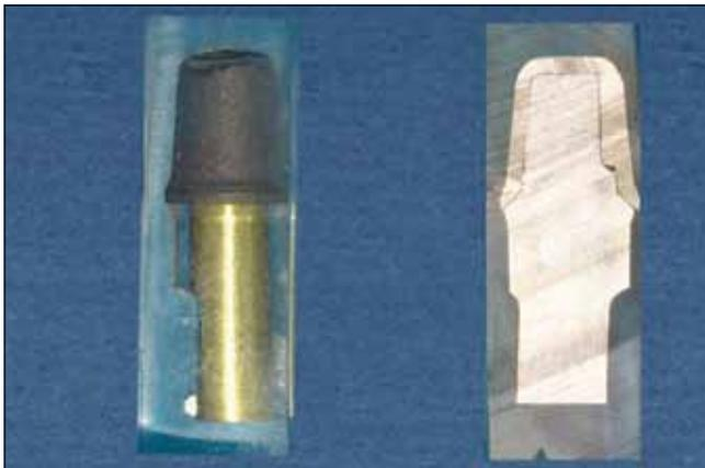
**Figure 3:** Specimen embedded in acrylic resin (Left). Longitudinal section of the specimen (Right)
