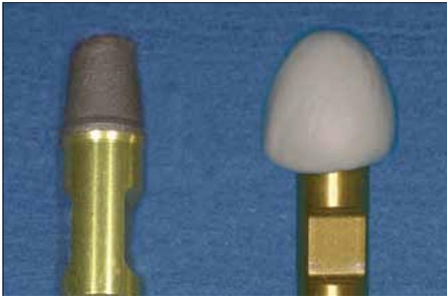
**Figure 1:** Cast frame fabricated as a model for other specimens (Left). Silicone index as a mold for preparing specimens (Right)
