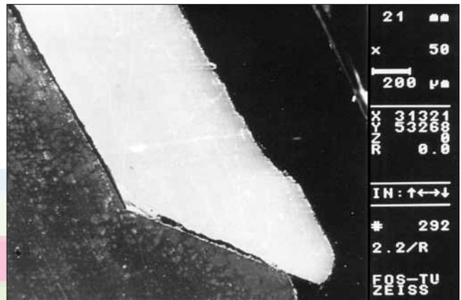
**Figure 9:** The SEM views of conventional wax-up in gold casting group (group 3n)
