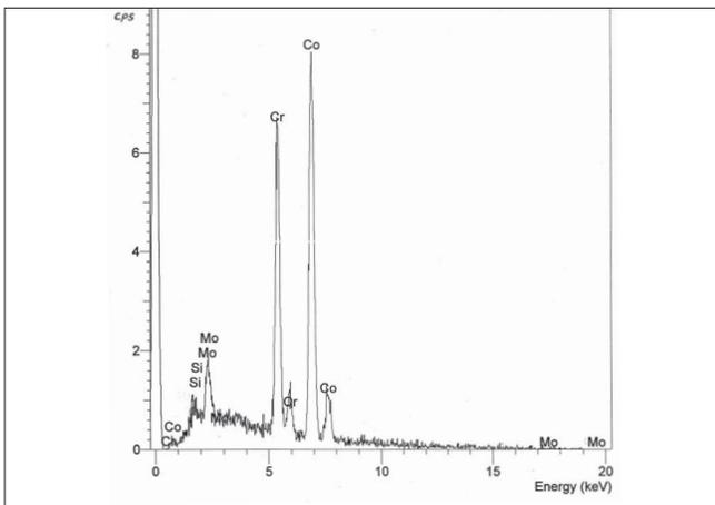
**Figure 2:** X-ray energy dispersive plot for uncorroded specimens
