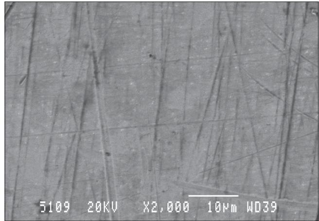
**Figure 4:** SEM photograph of polished specimen at 2000 × magnification
