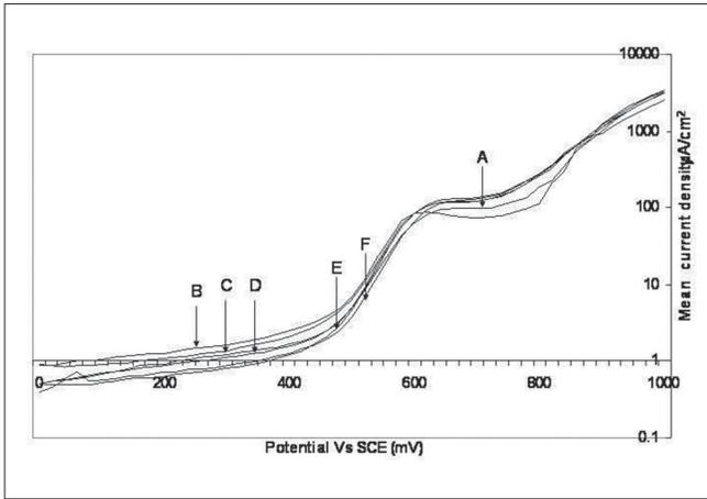
**Figure 1:** Anodic polarization curves of six generations. A- first, B - second, C - third, D - forth, E - fifth and F - sixth generations respectively
