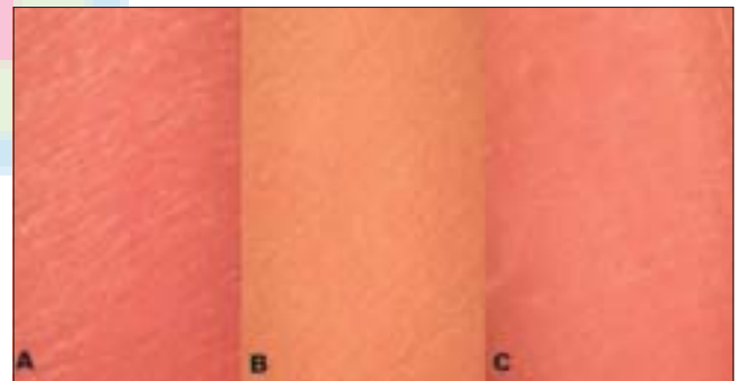
Figure 7: Adhesive fracture under light microscope for control group, A: Conventional heat cure denture base resin, B: High-impact heat cure denture base resin, C: Glass fiber-reinforced heat cure denture base resin
