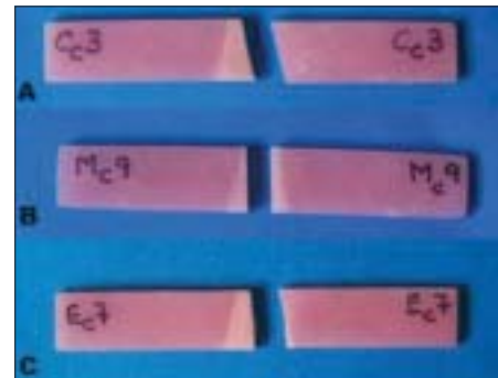
Figure 6: Fracture type — A: Adhesive fracture for control, B: Cohesive fracture for methylene chloride, C: Cohesive fracture for ethyl acetate
