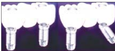
Figure 4: Representative diagram showing two implants supported fixed partial denture with elements and 6840 nodes showing two implants placed parallel to each other and (b) the other with one implant placed in 12° angulation to that of other
