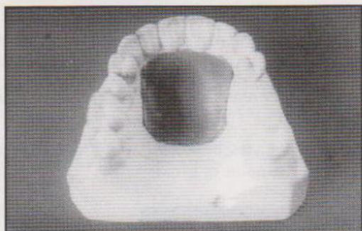
Fig. 4 : Wax flown over surface of foil pattern to reinforce it.
