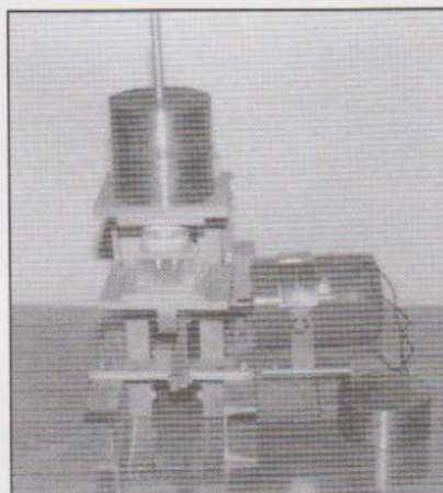
Fig. 3 : Jaw simulator with mounted dentures loaded with dead weights
