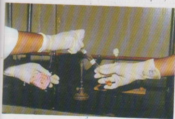
Fig. 2 - Impression disk is introduced into 10ml of T.S.B. in the test tube
