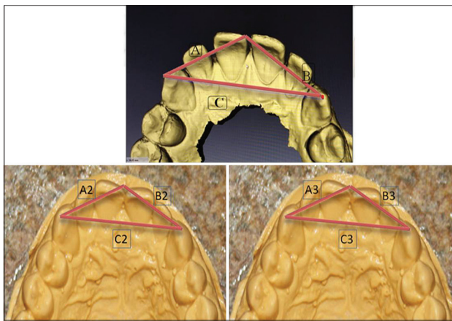
Figure 1: Reference points for measurements for dimensional accuracy
