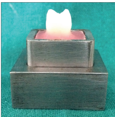
Figure 1: Mounted specimen in custom made metallic mold
