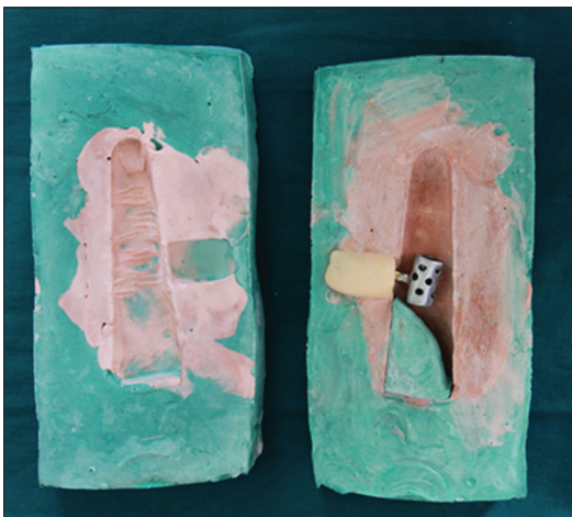
Figure 6: The dewaxed mold obtained with two-pour technique
