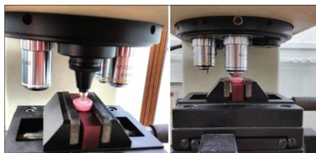
Figure 5: Samples mounted on Vickers indenter
