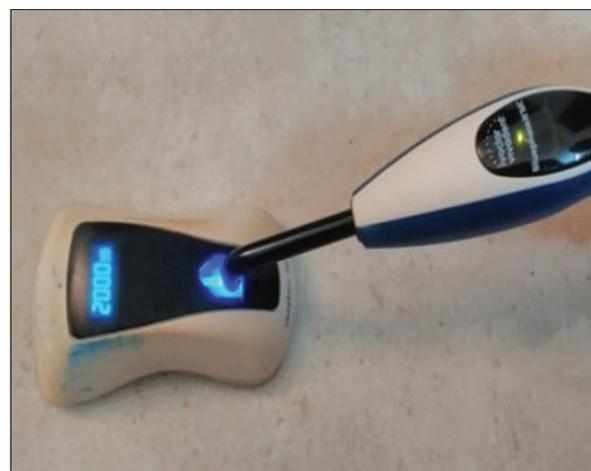
Figure 3: Radiointensity meter from Ivoclar Vivadent – to measure intensity or irradiance of light in mW/cm<sup>2</sup>
