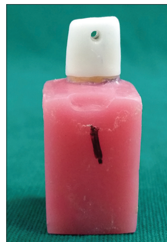
Figure 3: Milled zirconia coping with a hole
