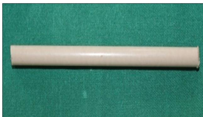
**Figure 1:** Poly-ether-ether-ketone ingot before milling
