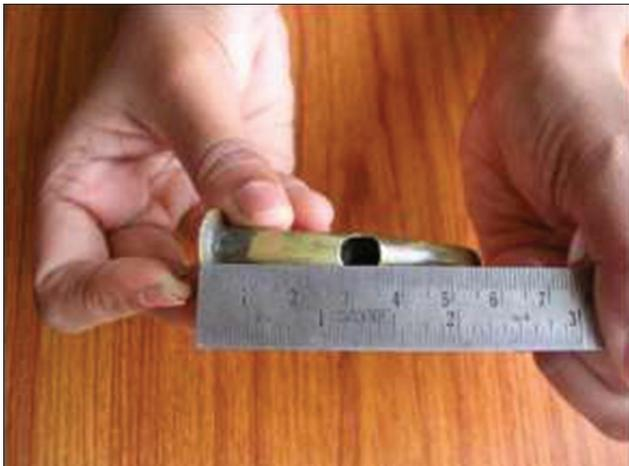
Figure 3: Length of old metal tube
