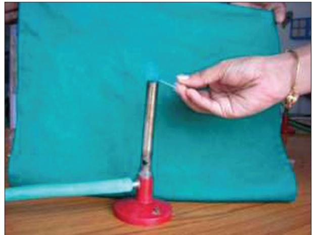
Figure 4: Polyethylene urethane sheet flamed
