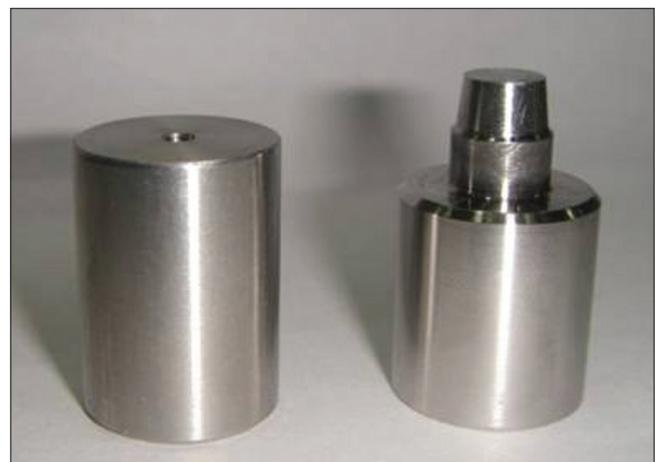
**Figure 1:** The customized stainless steel die assembly
