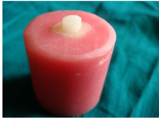
**Fig. 4** Zirconia rod bonded to dentin specimens using dual polymerizing self etching adhesive cement
