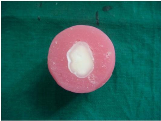
**Fig. 3** Tooth section mounted in auto polymerizing acrylic resin
