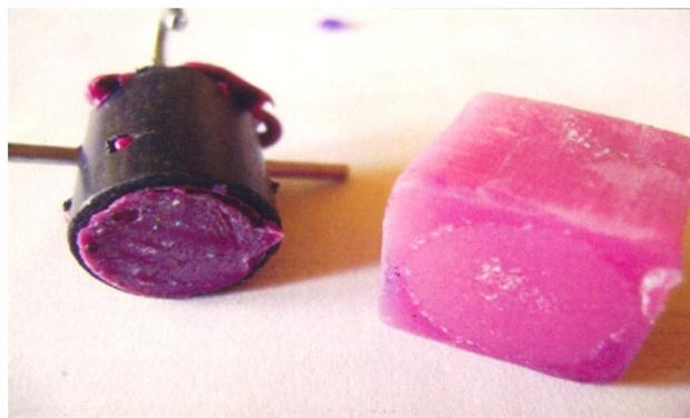
**Fig. 19** Debonded sample after tensile loading (Group B)
