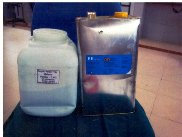
**Fig. 1** Materials for group A (autopolymerizing resin)
