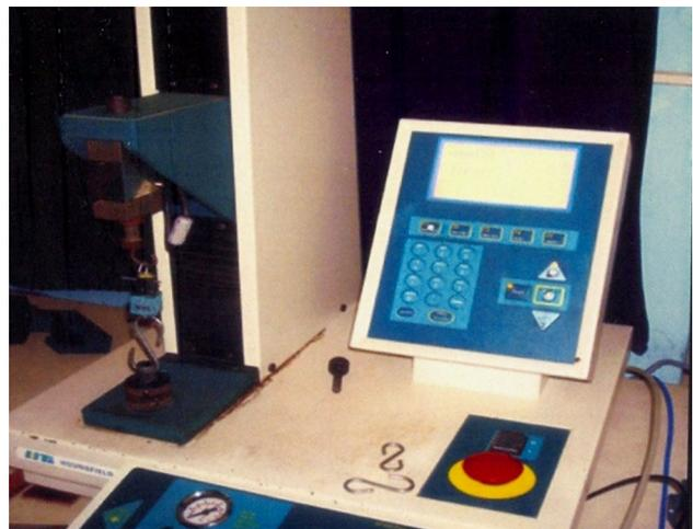
**Fig. 15** Group A sample attached to the universal testing machine
