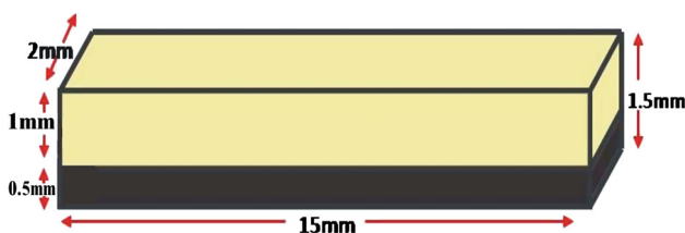
Fig. 1 Schematic figure of porcelain fused to metal bar samples
