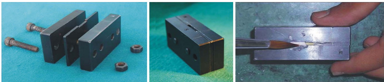
Fig. 3 Application of ceramic on metal bar using three piece customized mold
