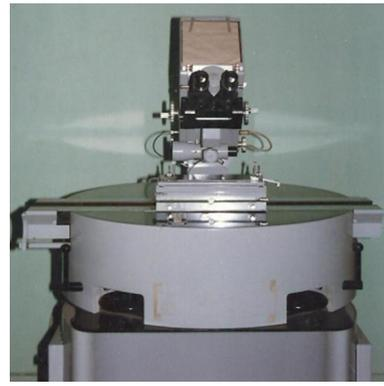
**Fig. 3** Measuring microscope (Resolution 1  $\mu$ m)
