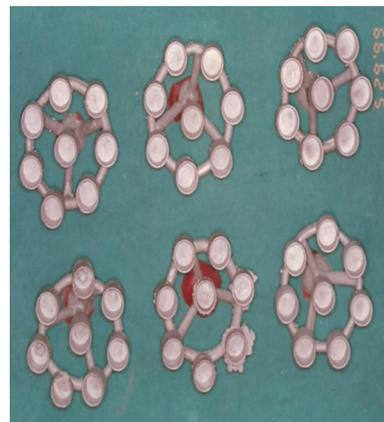
**Fig. 6** Metal frameworks showing various groups of castings
