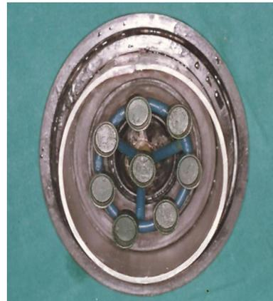
**Fig. 5** Wax patterns before investing attached to sprue former
