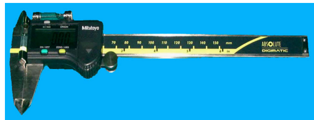
Fig. 1 Modified digital vernier caliper
