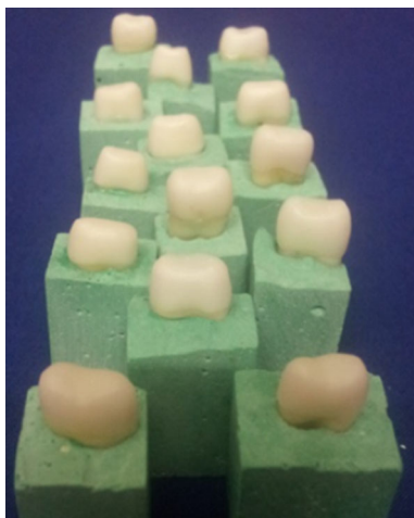
Fig. 2 16 Zirconia copings fabricated by Copy milling technique
