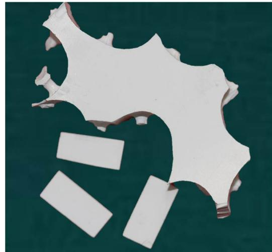
**Fig. 2** Commercially available pre sintered zirconia
