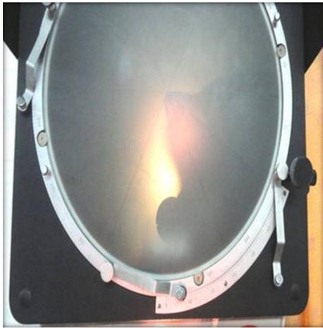
**Fig. 5** Profile projector measuring crown height from midpoint of ball bearing to tip of the cusp
