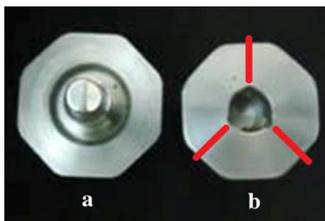
**Fig. 3** **a** Occlusal view of custom-made stainless steel model, **b** stainless steel former assembly showing 3 vertical slits
