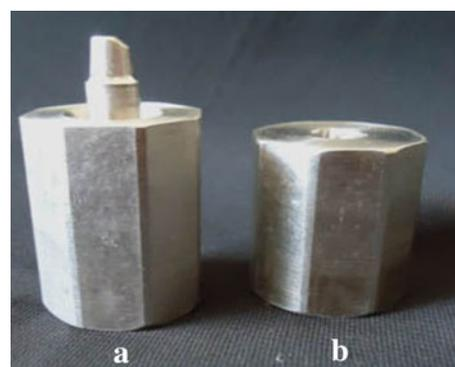
**Fig. 1** a Axial view of custom-made stainless steel model, b stainless steel former assembly
