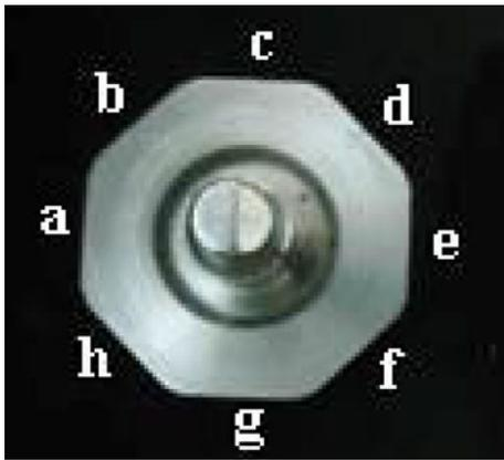
**Fig. 7** Schematic representation of 8 predetermined reference areas to be measured for vertical marginal gap
